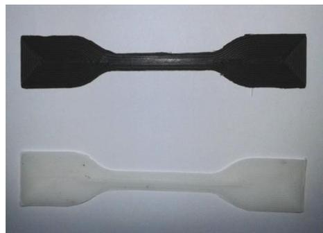
Figures a) 3D printing of a nanocomposite film b) Tensile test samples manufactured by 3D printing
